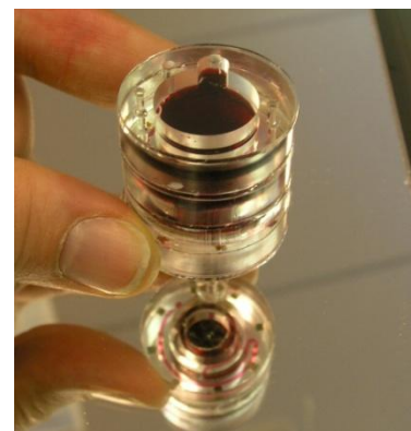
Figure 2: Modular micromechatronic and microfluidic environment for stimulating cardiac cells.
